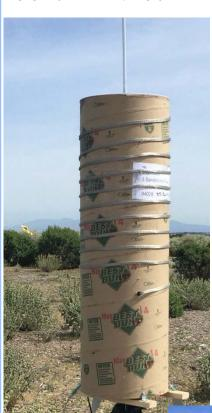
This odd looking thing is actually a pretty efficient 40-10 meter centerloaded high-Q vertical antenna made of a contractor's cardboard tube that was left over from my house remodeling project. had a SSB QRP QSO with a W9 station on 40m from Palo Alto's Baylands Open Preserve.
