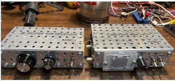
The receiver is a direct conversion CW receiver based on the Oct. 2021 QST article and the transmitter is the Tuna-Tin S based on the Dec 2020 QST article. Notice the translucent front dial cover of the transmitter is a repurposed hearing aid battery case.
