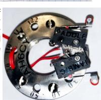
This one is made with two repurposed foreign coins sandwitching two microswitches.
