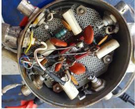
Antenna switching circuit in tuna can (antennas disconnected, turned upside down)
