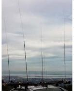
then hook up my AA-54 antenna analyzer and slide the rod in and out a few times to get each one tuned right – what a pain!. One day a rod fell out on the freeway, because I evidently hadn't tightened the two tiny setscrews, so I had to buy another Ham Stick!
