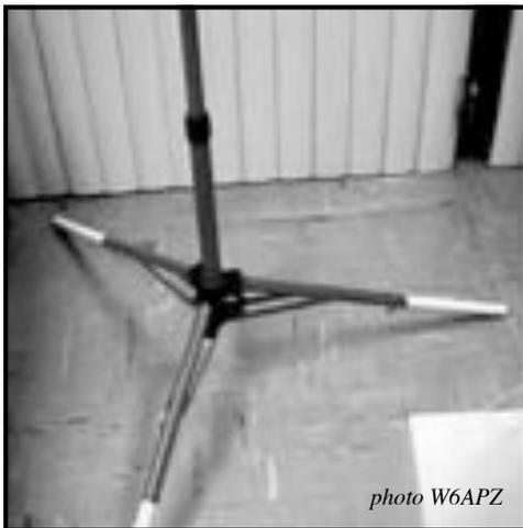
tripod in a windy environment. Another alternative if the tripod has been set up on earth would be to use a tent stake driven into the ground near each foot of the tripod, but secured to the PVC pipe.
