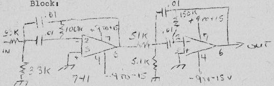
The first section has Q = 2.9 and a center f = 918 Hz.
