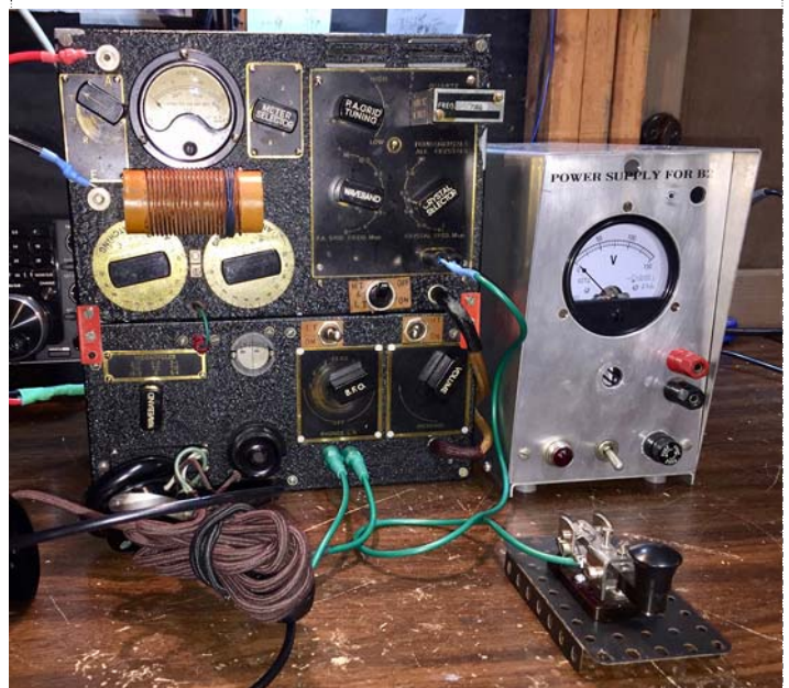
Fig 3. Restored B2 taken out of the metal box and put in an operating position
