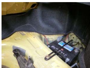
Fig 2: Miata Battery in Trunk
