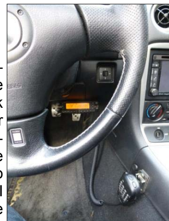
Fig 5: Head Unit mounted under dash
